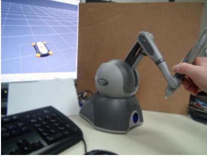
Fig. 3: PHANToM OMNI slave controller is used to control the youbot simulated using ROS
